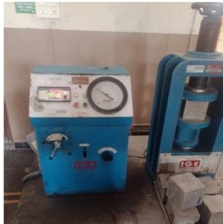
Compressive testing machine
